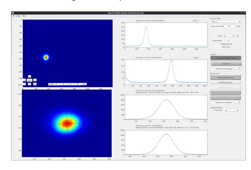
• Vertical beam size at source points is determined by a dispersion wave (which excites vertical emittance, a global conserved quantity) relying on 32 skew quadrupoles:
