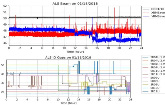
Figure 1: Electron beam size as measured the ALS diagnostic beamline 3.1 during a user run (top) showing roughly  $2.5 \mu\text{m}$  variation (5%) in the vertical caused by changes in vertical ID gaps (shown, bottom) and horizontal EPU shifts (not shown here).
