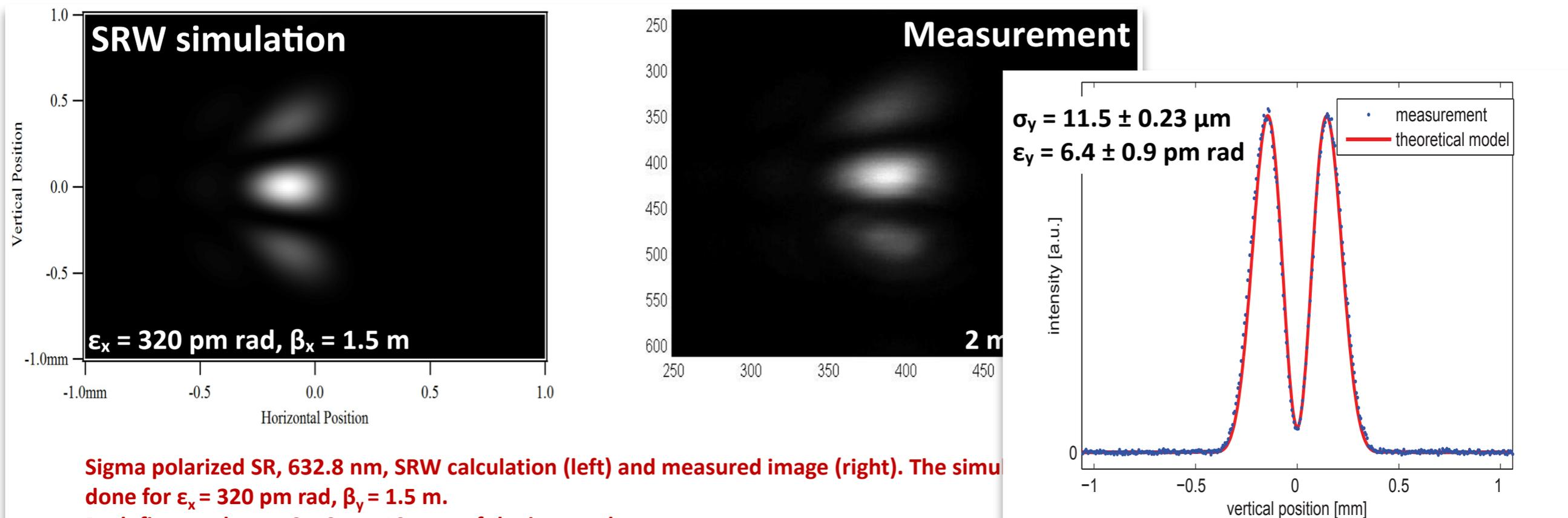
**Sigma polarized SR, 632.8 nm, SRW calculation (left) and measured image (right). The simulation is done for  $\epsilon_x = 320 \text{ pm rad}, \beta_x = 1.5 \text{ m}$ .**
