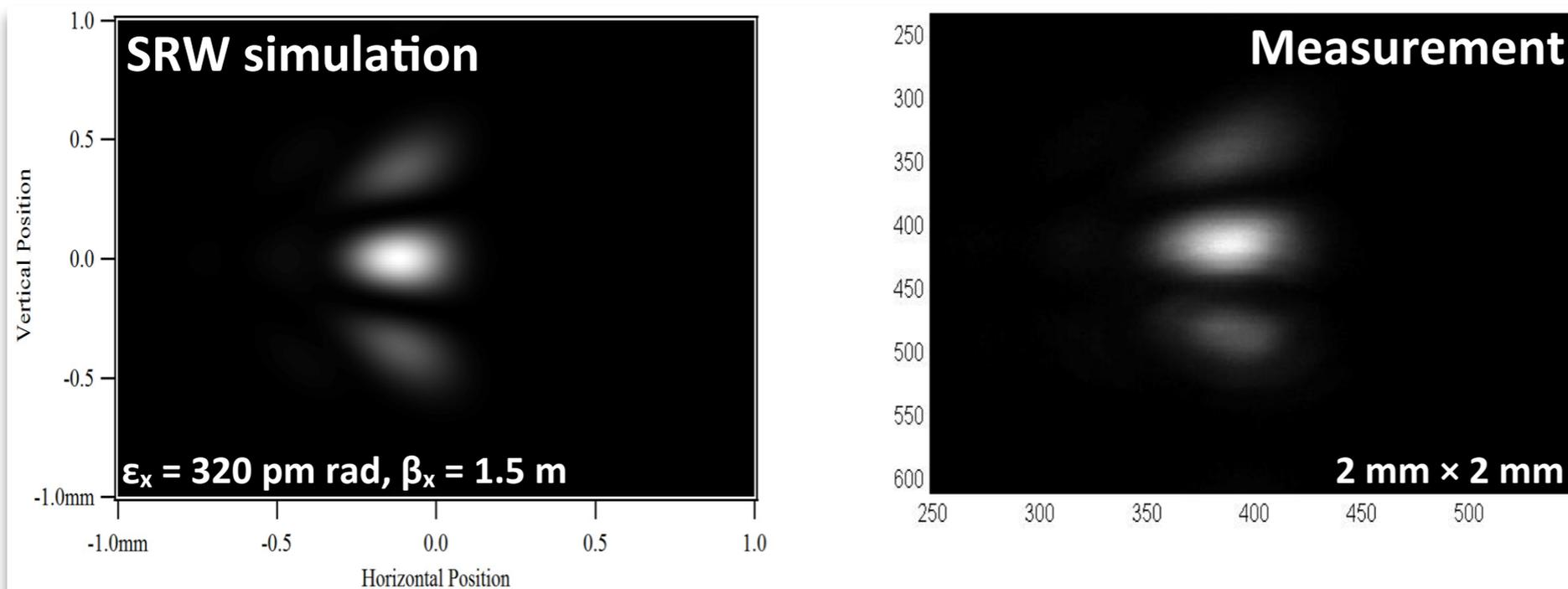
**Sigma polarized SR, 632.8 nm, SRW calculation (left) and measured image (right). The simulation is done for  $\epsilon_x = 320 \text{ pm rad}$ ,  $\beta_y = 1.5 \text{ m}$ .**
