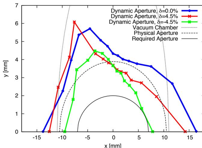
**Figure 5:** Dynamic aperture at the center of the long straight section in the MAX IV 3 GeV storage ring (bare lattice). Tracking was performed with Tracy-3 in 6D for half a synchrotron period. For comparison, the vacuum chamber and physical aperture (projection of vacuum chamber to the track point) are also indicated in the plot.
