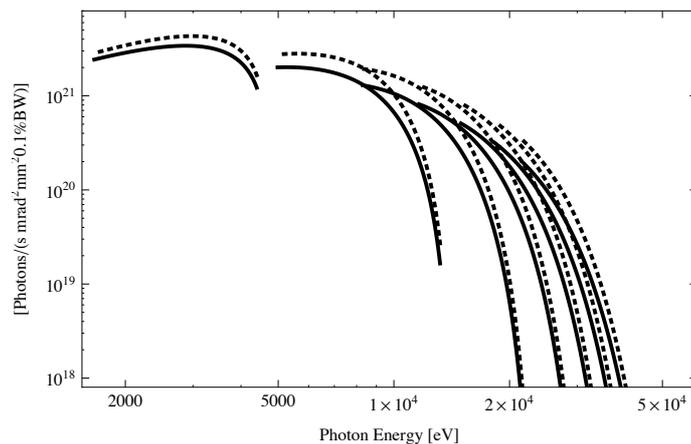
**Figure 8:** Spectral brightness at peak energy of a typical in-vacuum undulator installed in the MAX IV 3 GeV storage ring with 500 mA stored current and vertical emittance set to 8 pm rad (solid line) and 2 pm rad (dashed line) [26].
