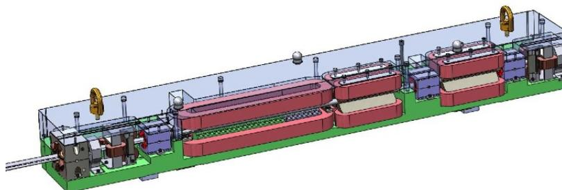
**Figure 6:** Drawing of a matching cell magnet block with soft-end gradient dipole, quadrupole doublet, defocusing sextupole (far left), three octupoles (blue), and two dipole corrector pairs.
