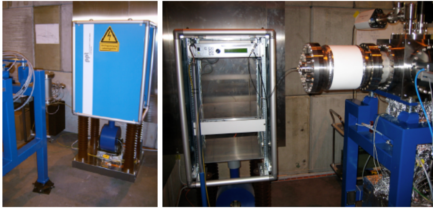
Figure 4.8: The hotdeck consisting of a 19" rack that holds the gate pulser and electronics for communication (in the rack) as well as the 230 V isolating transformer (between the rack and the base). The cathode flange with the SMA vacuum feedthrough, ceramic insulation and diagnostics cube are shown in the right picture.
