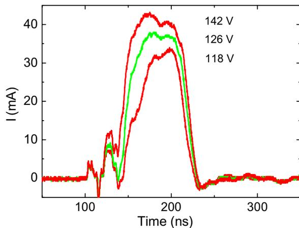
Figure 3: Collected current pulses for a SRI Inc. FEA with 50,000 Mo tips for 100 ns square applied voltage pulses of 118, 126 and 142 V.
