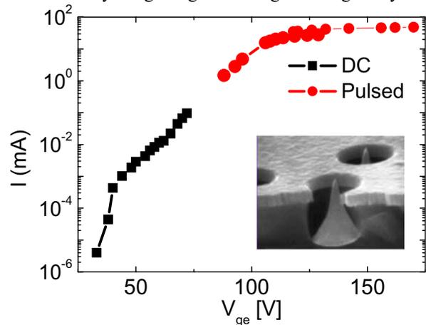
Figure 2: Current-voltage characteristic in DC and pulsed regime for a SRI Inc. FEA (1 μm diameter, 50,000 Mo tips) Insert: SEM picture of some conical Mo tips (SRI website [3]).
