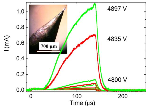
Figure 4: Collected current pulses for a single ZrC tip from APTEch Inc. for different 100  $\mu$ s square applied voltage pulses.
