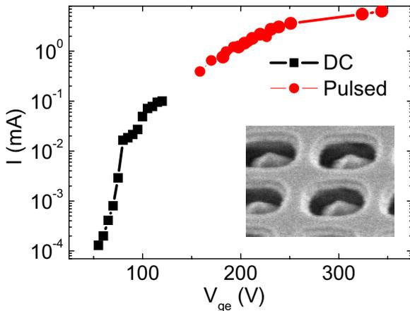
Figure 1: Current-voltage characteristic in DC and pulsed regime for a XDI Inc. FEA (170 μm diameter, 3,000 diamond tips). Insert: SEM picture of some pyramidal diamond tips.
