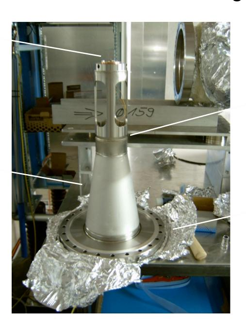
Custom welded feedthroughs
