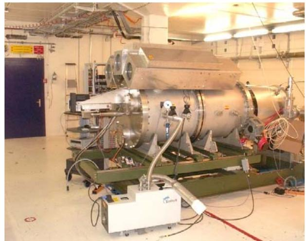
Figure 6. Installation of the 500-kV pulser in the test-bunker OBLA.
