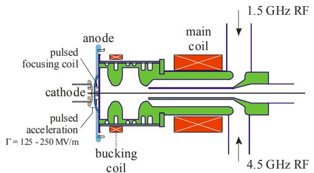
Figure 3. Layout of the high-gradient accelerating section followed by the initial RF acceleration [8].
