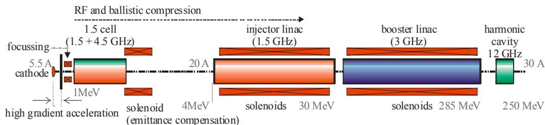
Figure 2. Schematic layout of the injector.
