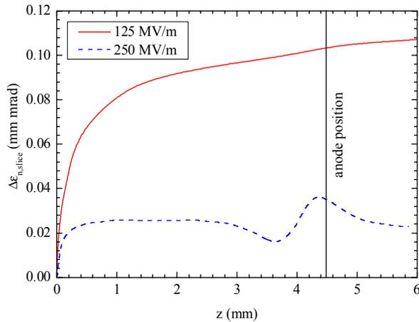
Figure 4. CAPONE [9] simulation of the slice emittance growth of a uniform electron bunch (Tab. 1) in a DC accelerator field (1 pC slice with an initial radius of 0.25 mm).
