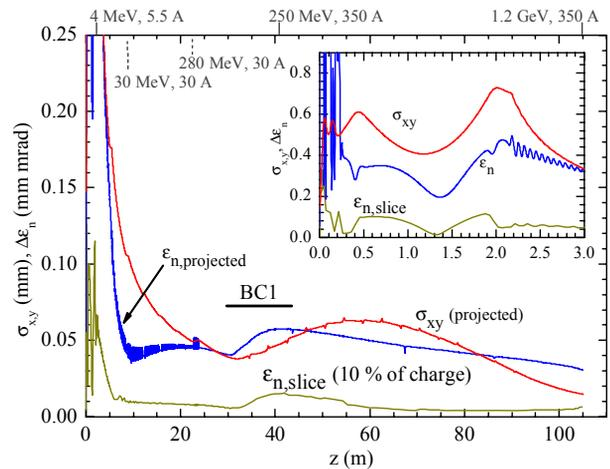
Figure 5. HOMDYN [10] simulation of the beam envelope and emittance dilution for the PSI FEL linac up to BC2, see Fig. 1. The inset is a zoom of the first 3 m.
