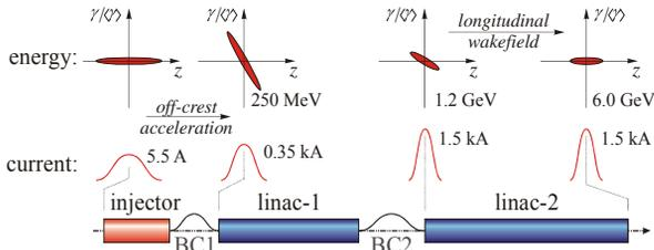
Figure 1. Functional layout of a low-emittance linac for an X-FEL. See text for details on the longitudinal shaping of the electron bunch.
