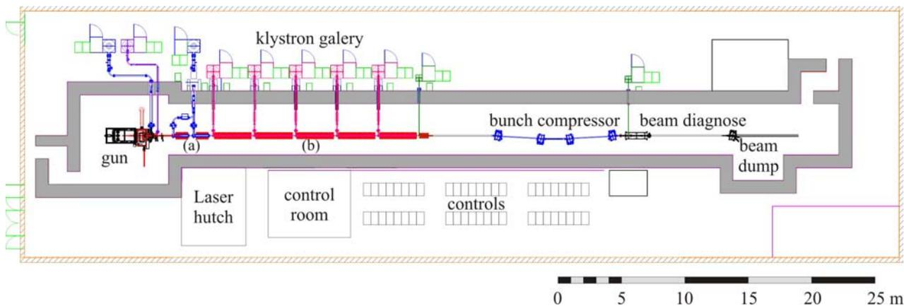
Figure 7. Layout of the 250 MeV test injector. The areas (a) and (b) mark the injector linac and booster linac as depicted in Fig. 2. The designed tunnel is sufficiently long to house the first bunch compressor (BC1 in Fig. 1).
