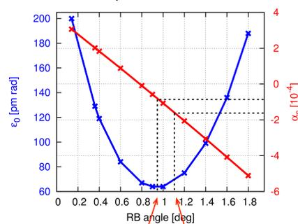
Minimum emittance  $\rightarrow$  quasi-isochronous. Detuned for sizable  $\alpha_c$  while retaining very low emittance
