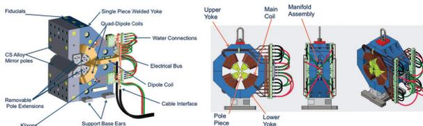
Figure 6: (Left) Design of the transverse gradient dipole which is being built as the first R&D magnet to demonstrate the critical technical features of ALS-U magnets. (Right) Design of the reverse bend quadrupole starting construction.
