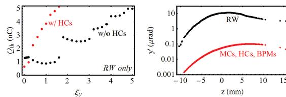
Figure 4: (Left) TMCI threshold as a function of chromaticity. (Right) Transverse wakefield kick due to resistive wall effect in small gap undulator chambers as well as selected other impedance sources.
