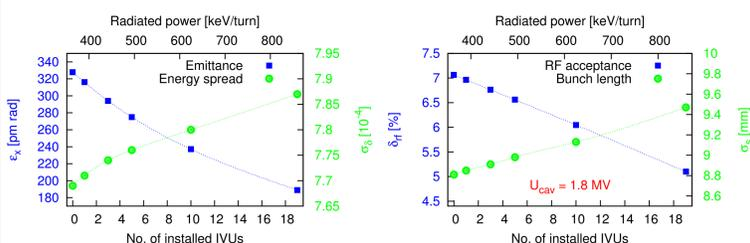
Beam parameters of the MAX IV 3 GeV storage ring as a function of the number of installed IVUs. At fully closed gap each IVU adds 26 keV/turn to the synchrotron radiation losses. Left: zero-current emittance and natural energy spread. Right: RF acceptance and zero-current bunch length assuming 1.8 MV overall cavity voltage.
