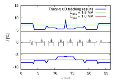
Lattice MA for one achromat of the MAX IV 3 GeV storage ring from 6D tracking with Tracy-3 using actual vacuum chamber apertures.
