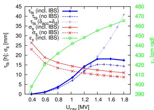
Touschek lifetime, bunch length, and horizontal emittance in the MAX IV 3 GeV storage ring bare lattice as functions of the RF cavity voltage. Stored current set to 500 mA, vertical emittance adjusted to 8 pm rad.
