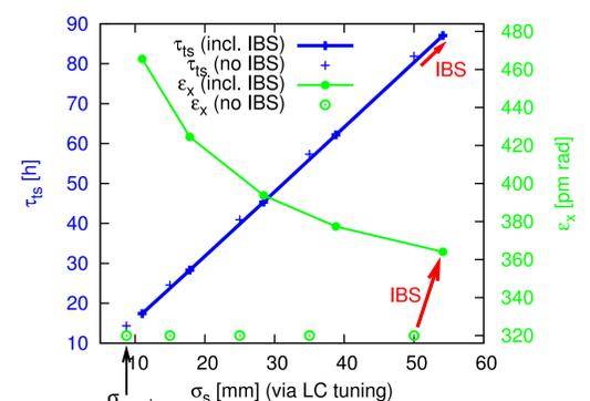
Touschek lifetime and horizontal emittance as functions of bunch length. Stored current set to 500 mA, vertical emittance adjusted to 8 pm rad. The calculated Touschek lifetime is based on resulting overall MA from tracking and actual vacuum apertures.
