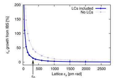
Horizontal emittance growth from IBS at 500 mA as a function of lattice emittance assuming the latter can be adjusted freely while keeping the energy spread constant. The overall MA has been set to 4.5% and the vertical emittance is always adjusted to 8 pm rad.
