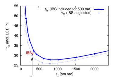
Touschek lifetime from 6D tracking with Tracy-3 as a function of equilibrium emittance assuming the lattice emittance could be adjusted freely while keeping the energy spread constant. The overall MA has been set to 4.5% while the vertical emittance is adjusted to 8 pm rad.
