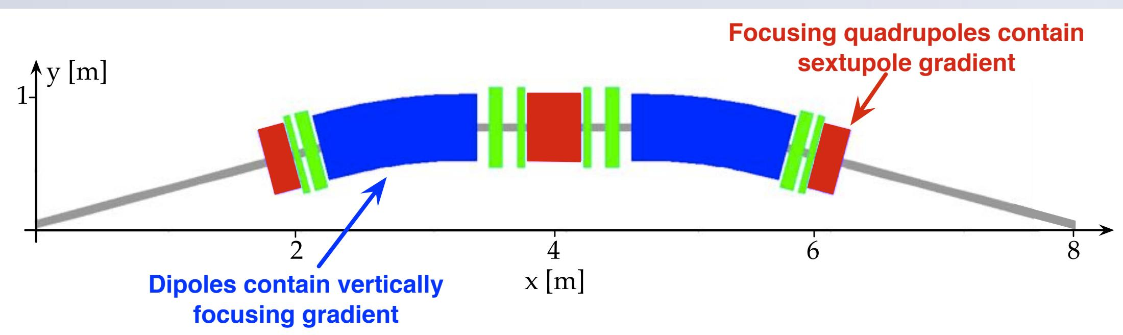
Combined-function magnets described in lattice by array of slices
