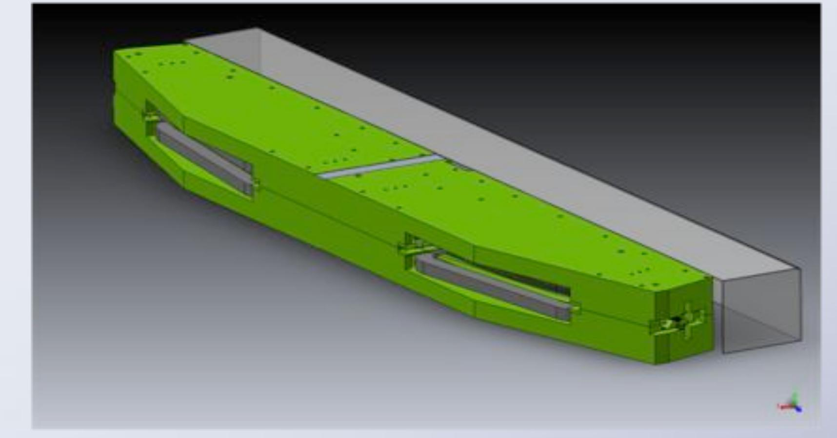
Entire DBA cell is machined from one solid iron block (demonstrated in MAX III).
