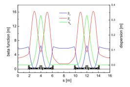
Figure 1: Two achromats with a 3.5 T SCW insterted in between.
