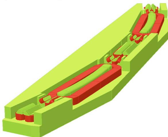
Figure 2: Magnet half block with coils in red [6].
