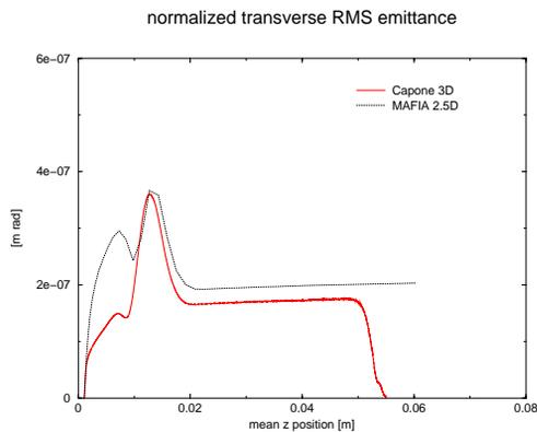
Figure 5: Total normalized RMS emittance  $\epsilon_x$  as a function of mean  $z$  position.
