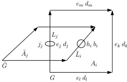
Figure 2: Topological structure of the Finite Integration Algorithm.
