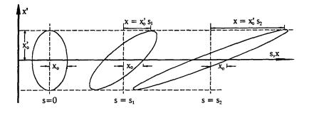
**b**) The initially diverging beam becomes convergent after passing the focussing lens. It converges until it reaches the beam waist where the beam size reaches a minimum (and the divergence reaches a maximum). From here on the beam becomes divergent again.
